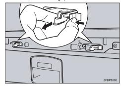
10 Lift the printer and move it to the place where you want to install it. When lifting the printer, use the pullout grips o the front side and the inset grips on the rear side. After that, push the grips into the printer.
